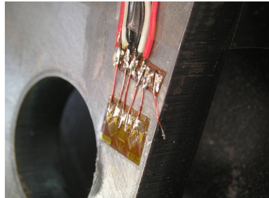
Figure 17: Strain Gauge glued on Main Plate
