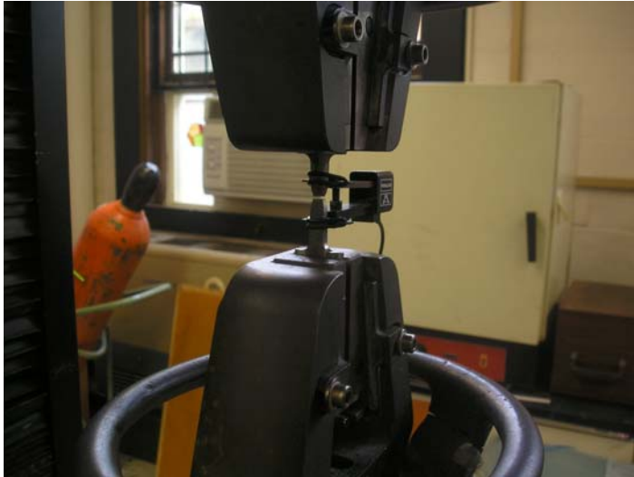
Figure 3: Fractured test specimen loaded in Instron Tester.
