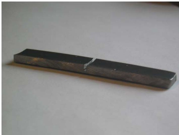
Figure 4: Impact test specimen fabricated from round pipe.
