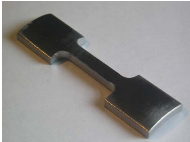
Figure 2: Tensile test specimen fabricated from round pipe.
