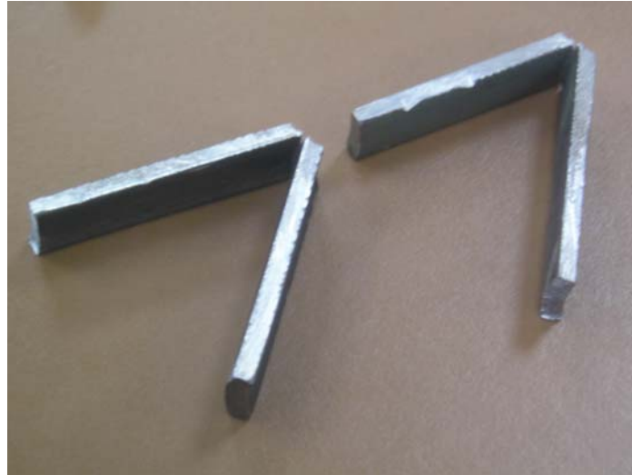
Figure 14: Appearance of impact specimens after testing.
