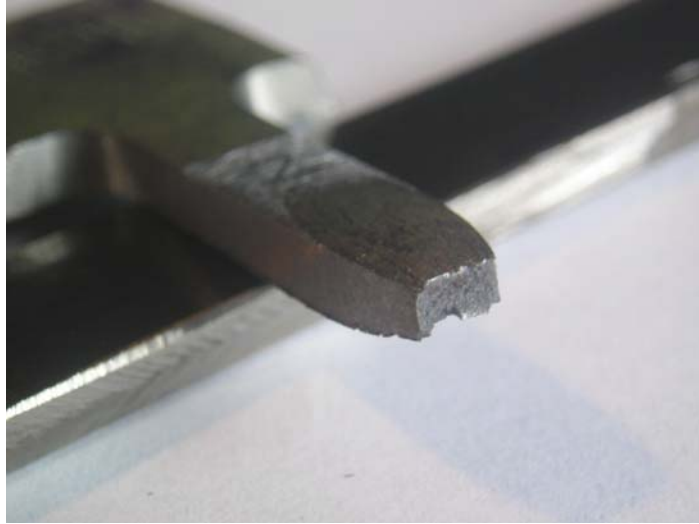
Figure 5: Cross section of specimen after necking and fracture.
